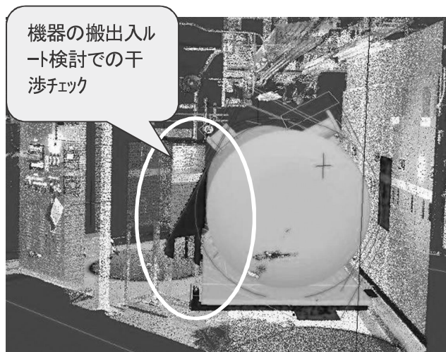
Fig. 3 Interface check of loading route of equipment
