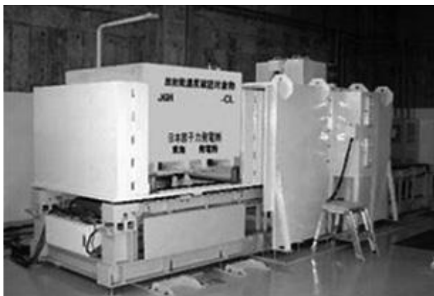
Fig. 23 Basket type clearance level measurement system 7)
