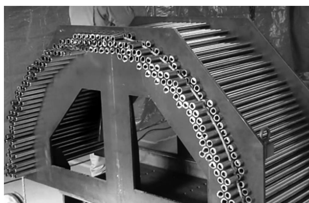
Fig. 14 Bandsaw cutting test of steam generator tubes
