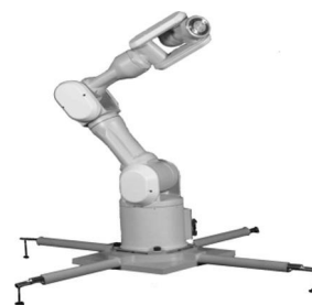
Fig. 9 7-axis manipulator (10kg capacity)
