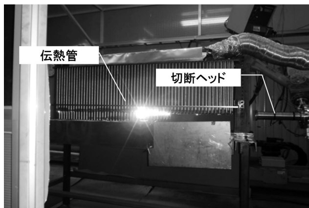
Fig. 13 Laser cutting test of steam generator tubes
